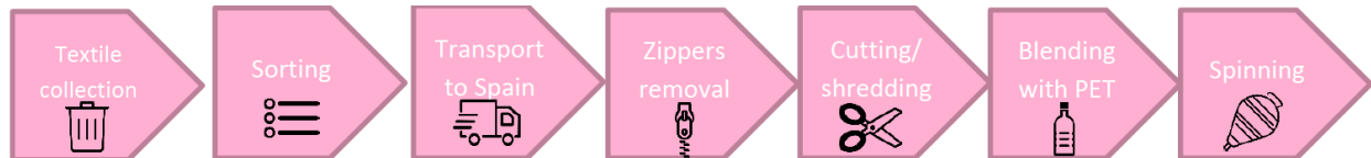
Figure 1: Production process ReBlend fibre
